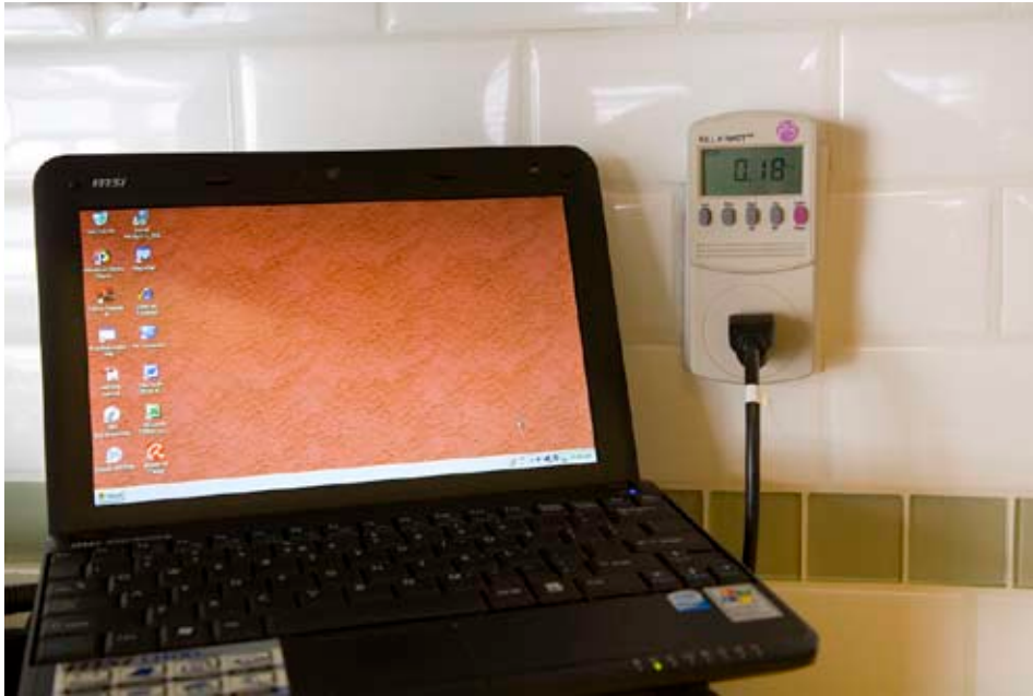
Energy monitors tell you how much electricity is being used by your plug-in devices.
