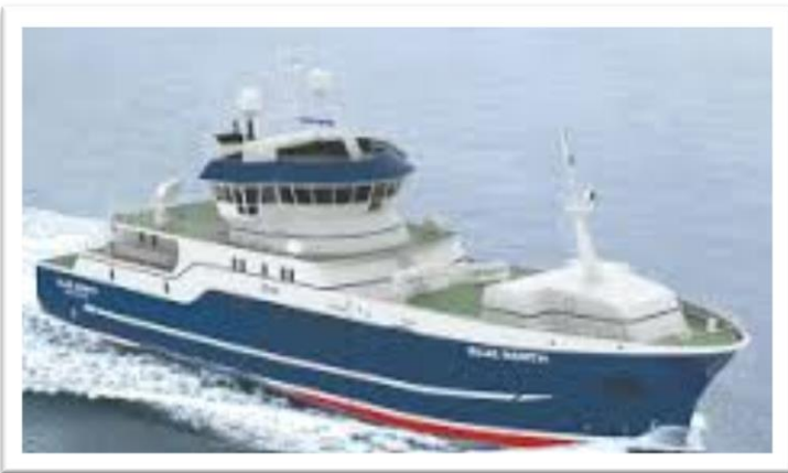
Dakota Creek is building a state-of-the art environmentally friendly fishing vessel for line-caught cod. The design keeps weight low, making the ship 30% more fuel efficient. Credit: Blue North.
